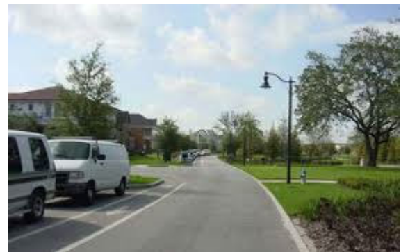
The addition of a bike lane and/or a parking lane on this street helps create a narrow travel lane for motorists.
