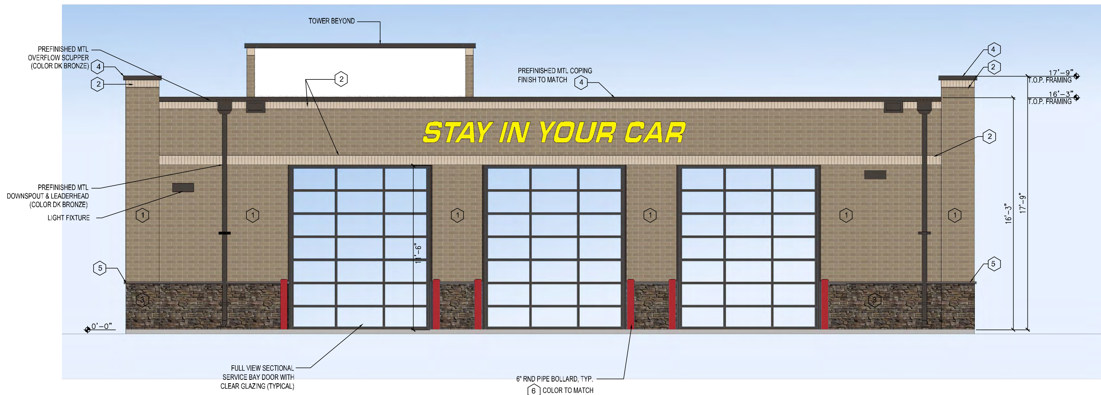
1 NORTH ELEVATION (PARKING) 1/4"=1'-0" OVERALL WALL AREA = 972 SF AREA OF STONE & BRICK = 624 SF (64%) AREA OF GLAZING = 348 (36%) SIGN AREA = 27.89 SF
