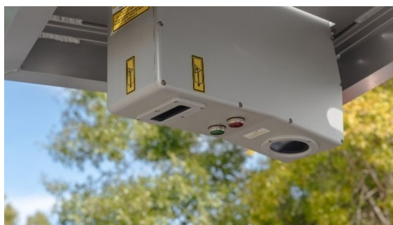
LCMS-2 Pavement Imaging System
