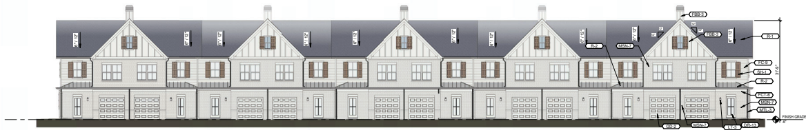
10 UNIT TOWNHOUSE - FRONT ELEVATION SCALE: 1" = 10'-0"
